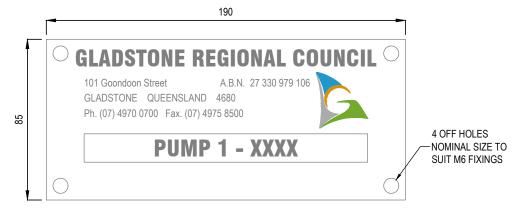
2mm Thick S/Steel Engraved; Black Text; Colour Logo; Pump Labels To Be Placed On Underside Of Pump Lids Above Each Pump
